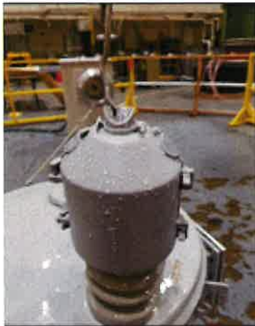
Wet Power Frequency Flashover Test
